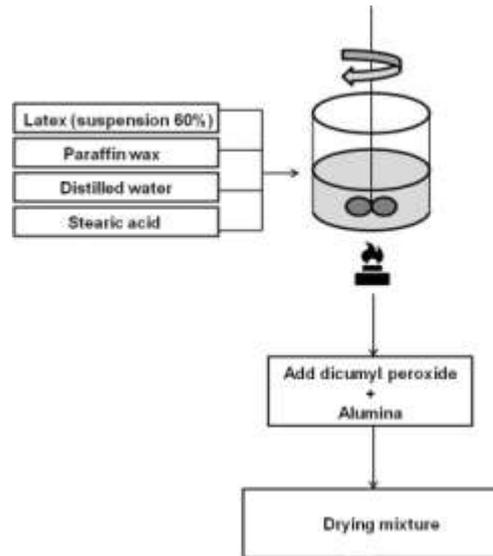
Fig 1: Method 1 (M1) of feedstock mixing.
