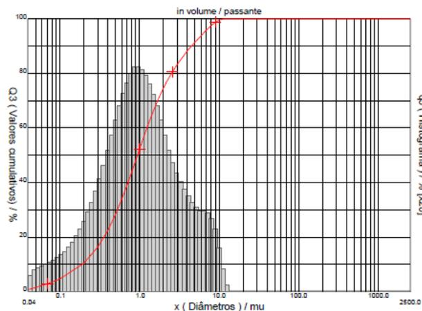
Fig 2: Alumina A-16 SG powder particle size distribution
