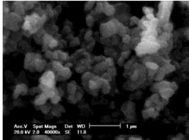
Fig 3: Morphology of the alumina powder.
