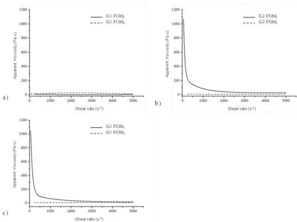
Fig 4: Viscosity vs. shear rate curve a) (L1P1) M1 e (L1P1) M2, b) (L2P3) M1 e (L2P3) M2 e c) (L1P2) M1 e (L1P1) M2.
