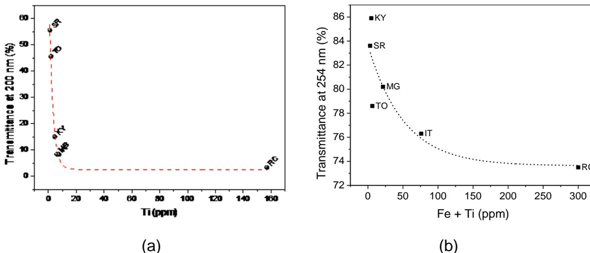
Figure 3. Effect of main metallic impurities on transmittance: (a) Ti at 200 nm and (b) Fe + Ti at 254 nm.
