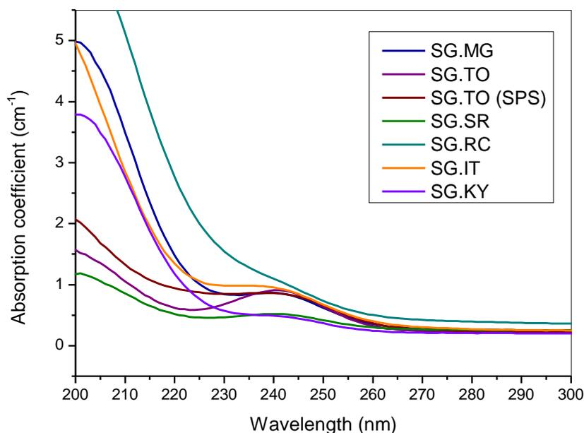
Figure 2. Absorption coefficient in the UV spectral range.
