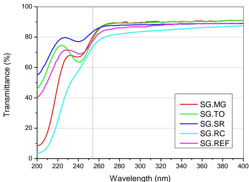
Figure 4. Comparison of optical transmittance of Brazilian quartz produced silica glasses with a commercial silica glass (SG.REF).
