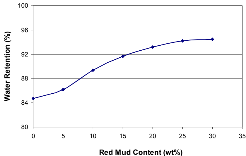
Figure 4. Water Retention of mortars as a function of red mud content.
