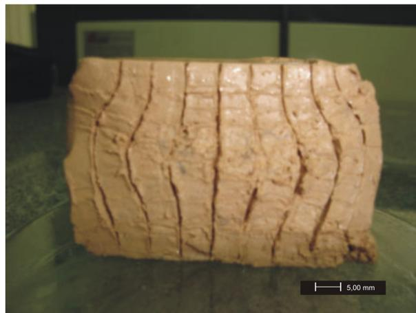
Fig. 2. Sectioned sample showing strain lines representing the stress distribution
