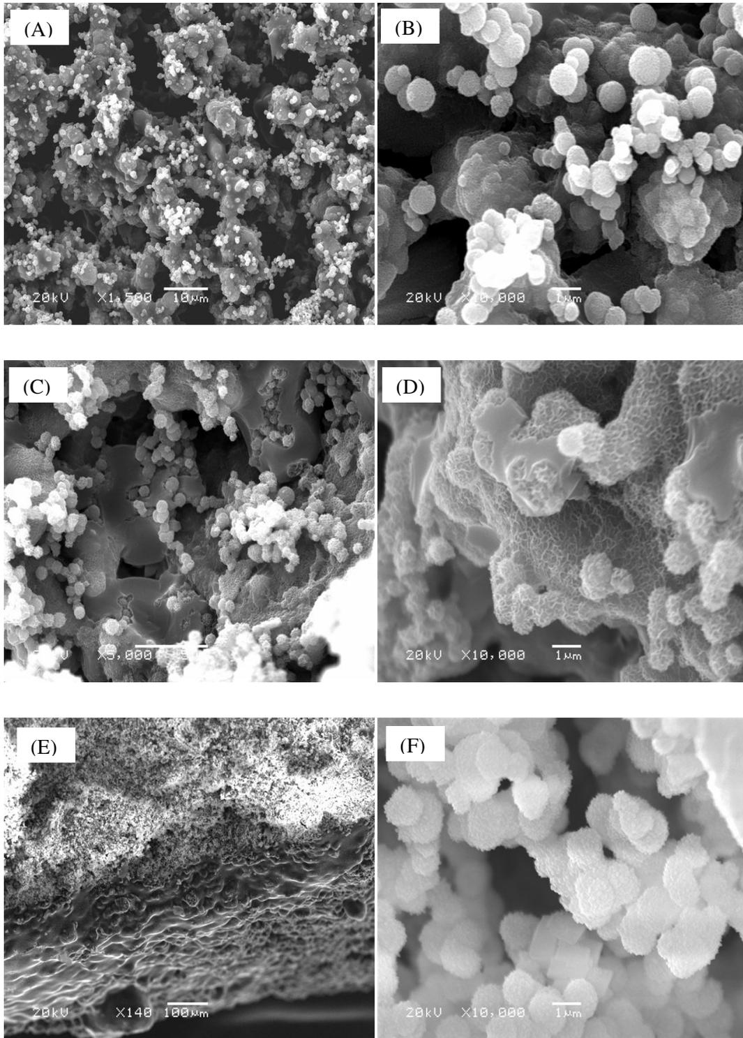
Figure 3. SEM micrographs of the surfaces of  $\text{Ca}_3\text{SiO}_5$  paste after soaking in SBF solution for 1h (A, B), 1 day (C, D) and 7 days (E, F).
