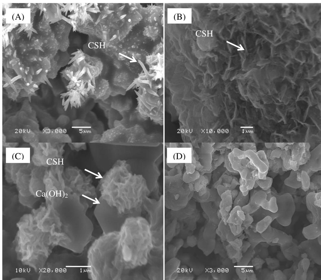
Figure 2. SEM micrographs of the surface and fracture surface. (A), (B) and (C) surface; (D) cross section.
