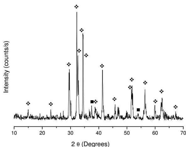
Figure 1. X Ray X-Ray diffraction patterns of  $Ca_3SiO_5$  powder. ❖  $Ca_3SiO_5$ , ■  $CaO$ .
