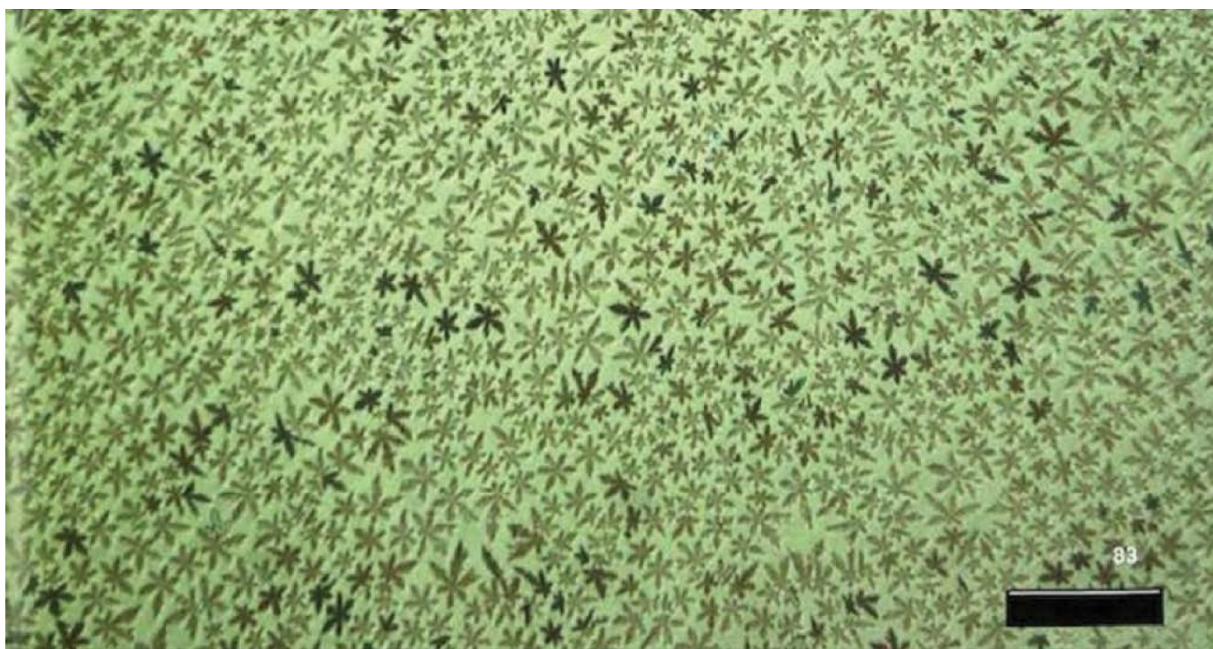
Optical micrograph showing a plethora of lithium metasilicate crystals embedded in the residual matrix of a rare (nucleant-free) glass-ceramic. The bar indicates 100 micrometers.
