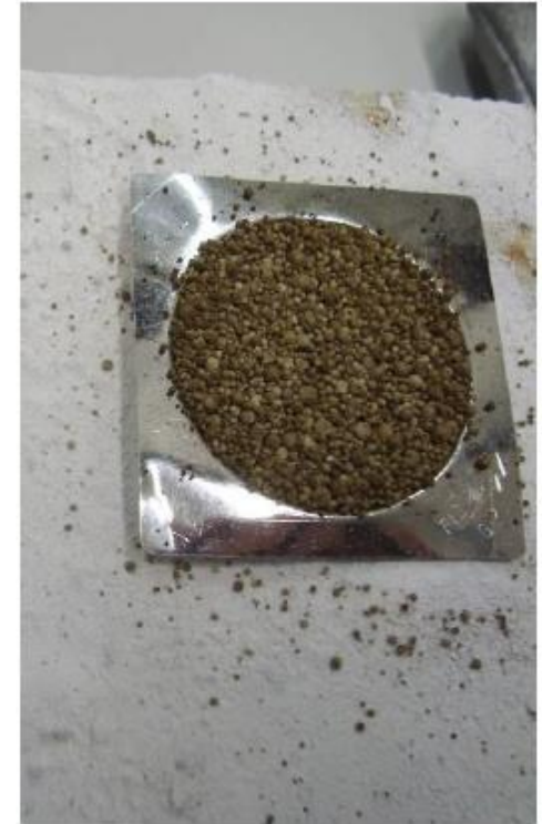
Example of a decrepitation test for dolomite
