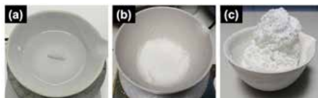
Figure 1: Images for a schematic description of the main steps in solution combustion synthesis (SCS).
